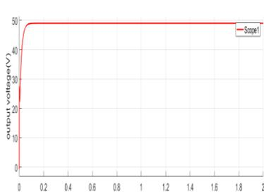
Output Voltage for step up converter constructed with KY and buck-boost converter
