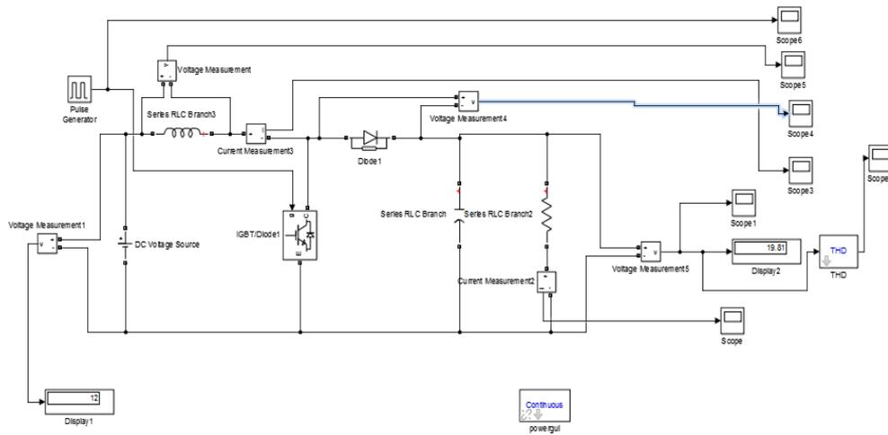
Simulation dia. for the Boost Converter
