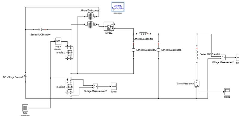
Simulation Diagram for the step up converter constructed with KY and buck-boost converter
