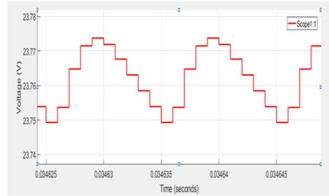
Output Voltage ripple for boost converter
