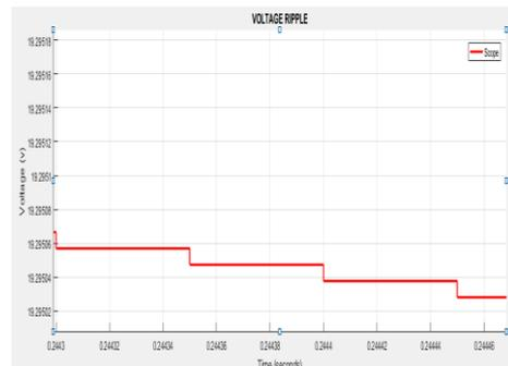
Output voltage ripple for KY Converter
