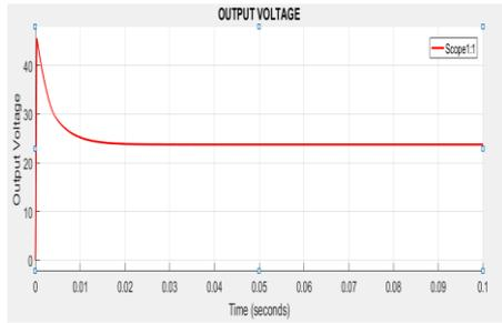
Output Voltage for boost converter
